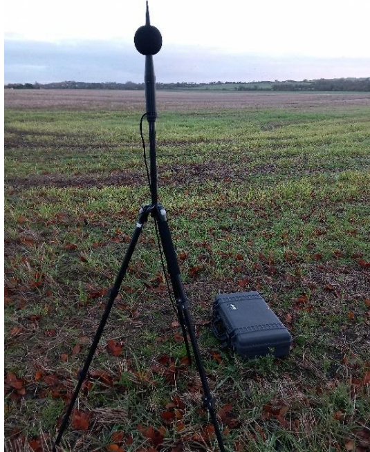
Figure 8: Attended noise monitor setup.
